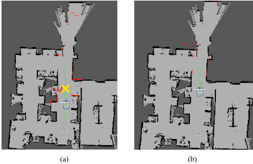
Figure 11.28: The navigation of the robot before (a) and after (b) the laser permanent failure (an X marks the moment in the robot's path when it occurred) and the reconfiguration from the main design to the kinect. The red dots correspond to the range scan reading of obstacles. Note the lack of lateral references due to the narrower angle span when in the kinect configuration.
